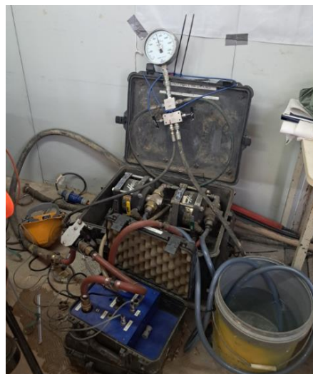
Plate 8: Set Up of the Hydraulic Pumps for O-cell
