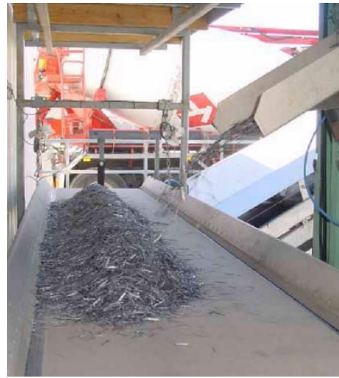
Figure 4: Conveyor belt for steel fibres
