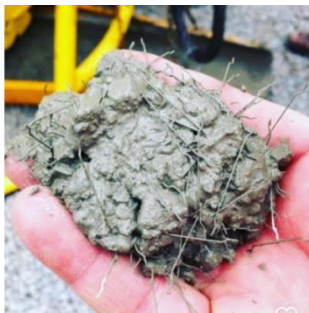
Plate 2 - Steel fibres in wet concrete
