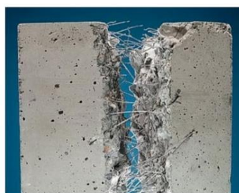
Plate 4: Post-crack behaviour of SFRC
