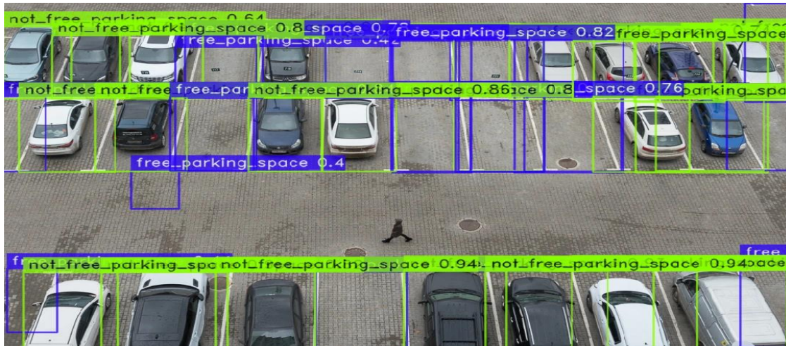
Fig 1: Parking Space Detection using Smart System [3]
