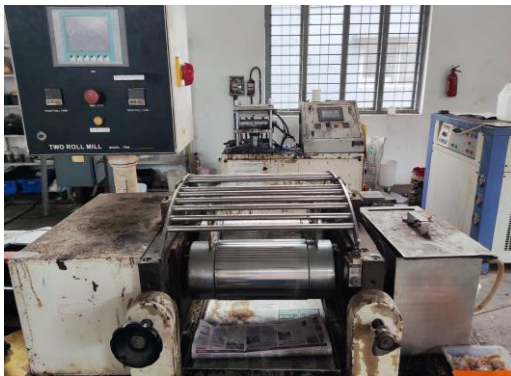
Figure 4: Two-roll mill mixer used for uniformly blending PLA and bagasse powder
