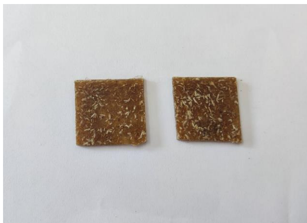
Figure 11: Density test samples made from PLA and sugarcane bagasse composite.
