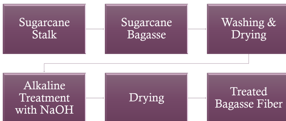
Figure 3: Flowchart which depicts the treatment of Sugarcane bagasse.
