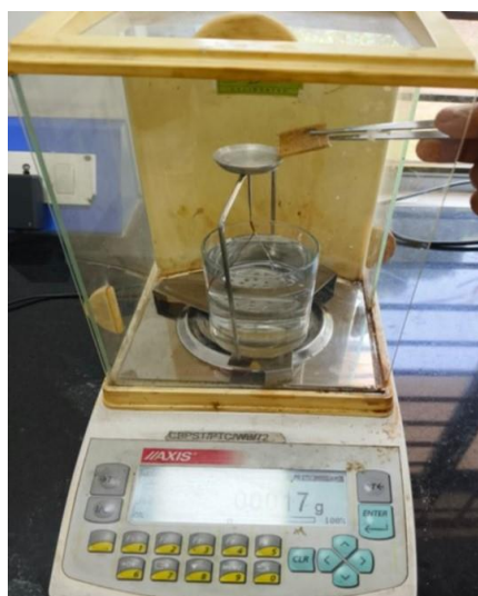
Figure 8: Density test apparatus used to determine the material density using the water displacement method.
