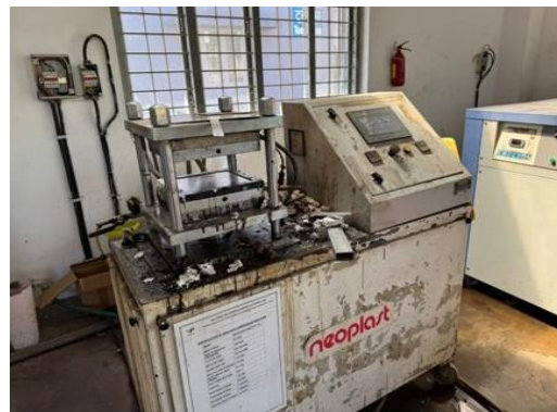
Figure 5: Compression moulding machine used to form composite specimens
