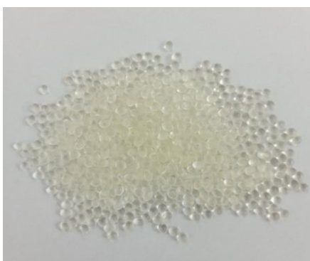
Figure 1: Granular form of Polyactic Acid (PLA), serving as the polymer matrix in the composite
