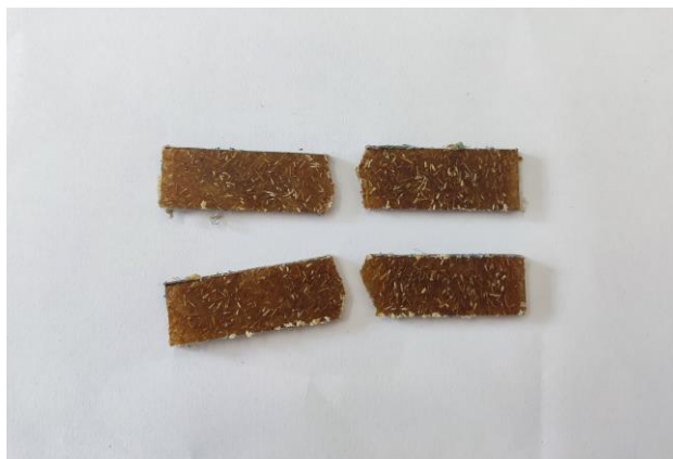
Figure 10: Impact test samples made from PLA and sugarcane bagasse composite.
