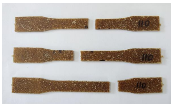
Figure 9: Tensile test samples made from PLA and sugarcane bagasse
