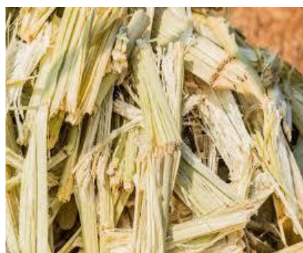
Figure 2: Raw Sugarcane Bagasse, a lignocellulosic agricultural by-product used as reinforcement in the composite
