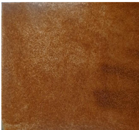
Figure 6: PLA & Sugarcane bagasse specimen formed after compression moulding
