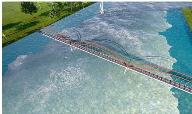
Fig. 18. 3D Model of vertical hanger bowstring bridge
