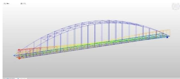
Fig. 11. Deflection diagram of vertical hanger bowstring bridge (isometric view)
