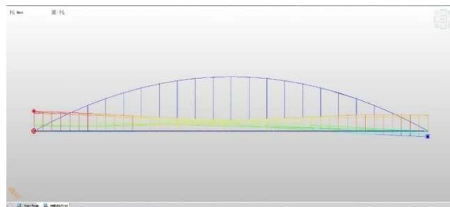
Fig. 14. Bending moment diagram of vertical hanger bowstring bridge
