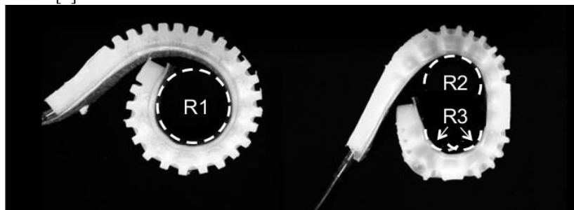
Fig. 1. Radius of curvature R1 during bending for an actuator designed with variable stiffness, was larger than R2 and R3 for a conventional actuator [4].
