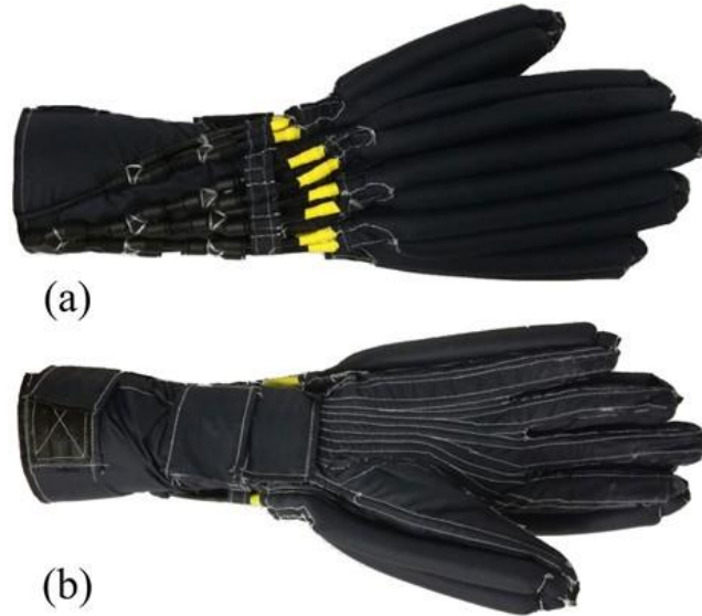
Fig. 4. Nylon fabric and latex bladder-based AirExGlove (a) hand dorsal side (pneumatic chambers pressurized), (b) hand palm side (tendon channel seams visible in white) [7].
