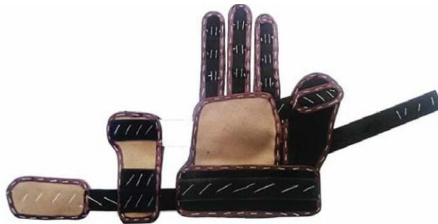
Fig. 3. The prototype of a fabric-based soft glove [6].
