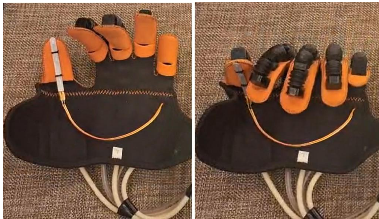
Fig. 8. Soft Exoskeleton Glove under actuation for all fingers
